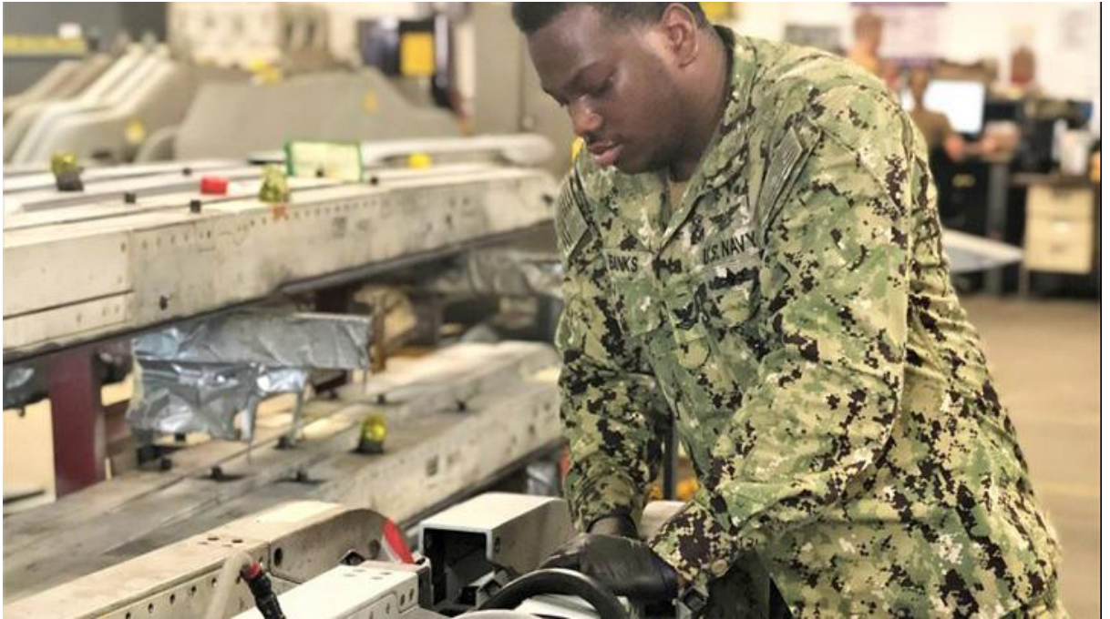
Petty Officer 3rd Class Kaylen Brooks, an aviation electronics technician, re-assembles a Multi-Purpose Color Display Unit in the Consolidated Automated Support Systems work center at Fleet Readiness Center West.
