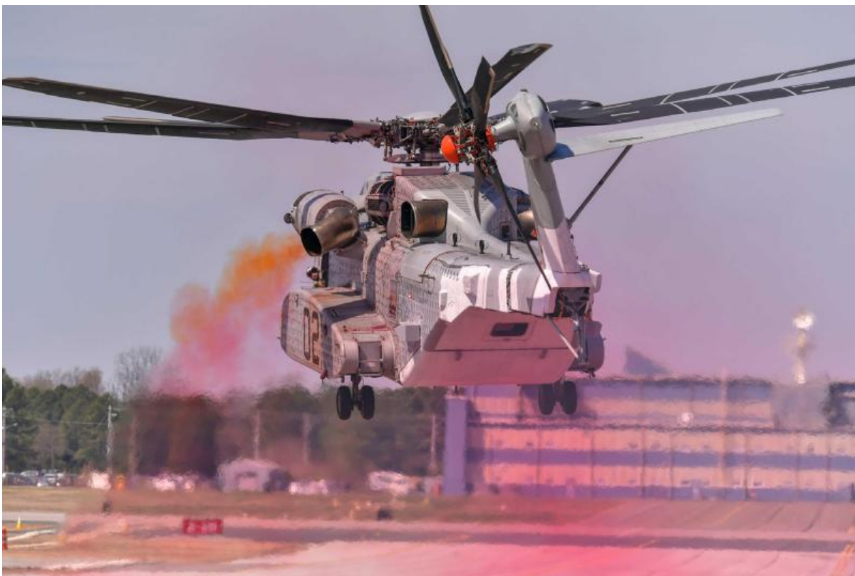
Colored oil smoke indicates rotor wake and wind effects while external “tufts” adhere to the outside of the CH-53K King Stallion showing surface airflow.
