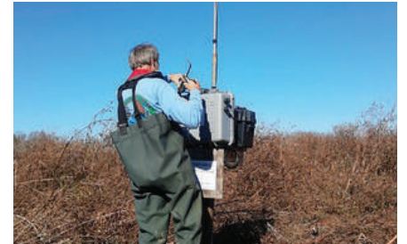
Researcher installing stationary radio receiver in the field
