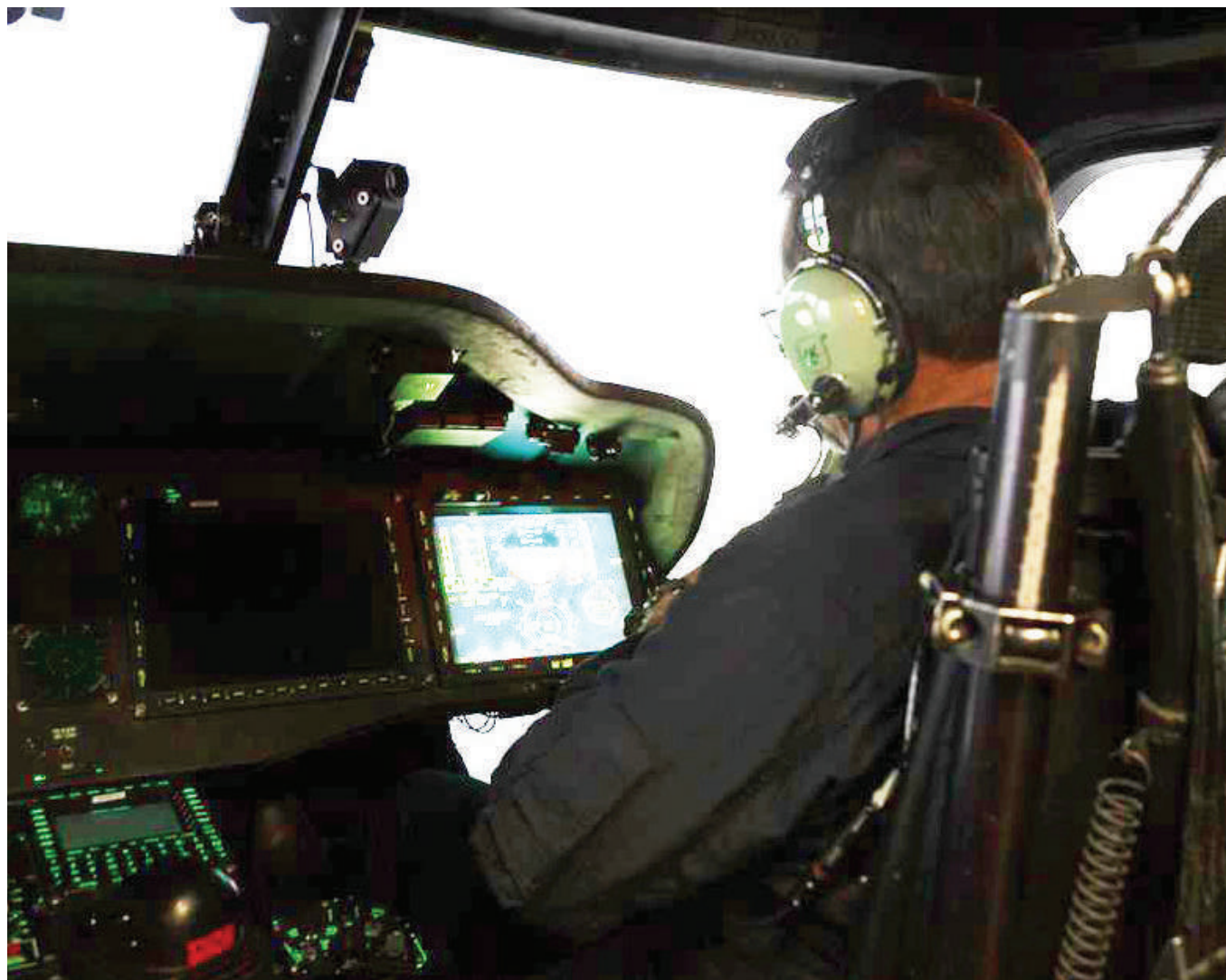
A rotary pilot performs a shipboard-landing maneuver through fog in a simulated scenario at the Naval Air Warfare Center Aircraft Division's Manned Flight Simulator in Patuxent River, Md. The pilot successfully landed his MH-60S on a virtual carrier in zero-visibility conditions using new landing aid software developed at the warfare center. A zero-visibility landing is an impossible feat in today's Seahawk helicopters where rotary pilots have no visual landing aids to assist with one of aviation's most difficult tasks. (U.S. Navy photo by Theresa Thomas)
