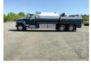
Vermeer D24x40 Navigator 2005 MACK Fuel & Oil Service Truck 2000 Gal Deisel tank & waste oil tank
