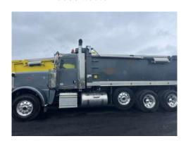
Two 2020 and one 2019 Peterbuilt Tri-Axle dump trucks. All have 20 front and 44 rears. 20 steerable lift axle Cumming IX 565 with Allison automatic transmissions. Two have steel bodies and one has aluminum
