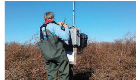
Researcher installing stationary radio receiver in the field
